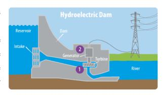
The rotating turbine rotates converts this mechanical energy into electrical energy using the generator. As a result, the potential energy stored into the reservoir water is initially converted into mechanical energy (via turbine) which is ultimately converted into electrical energy that we are so fond of. What if I told you that something similar takes place inside all living things!
